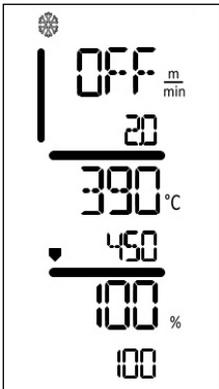
After finishing the welding work, switch off the heating with the **Heating "On/Off" button (31)**.
